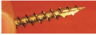
▲ A sharp point and long clearance flute help prevent splitting without piloting
